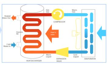
BALIEF make Innovative Heat Pump Provides four times more output (i.e. 1 unit of electricity input = 4 unit of heat output)
